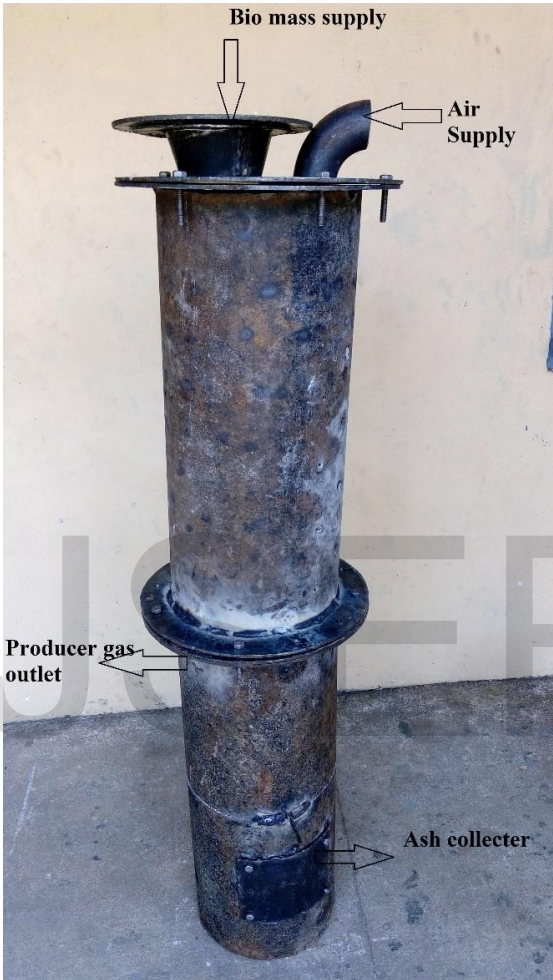
Fig. 1 Photoview of downdraft gasifier
